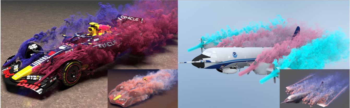
**Fig. 1.** Left: smoke (large) passing a racing car and its vorticity field (small). Right: smoke (large) passing an aircraft with 4 rotating propellers at a 15-degree angle of attack and its vorticity field (small). The wingtip vortices are captured by our algorithm in the vorticity field. Effective resolutions are  $512 \times 512 \times 1024$  on our adaptive grid implemented on GPU.
