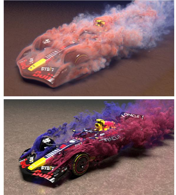
**Fig. 13.** Racing car, vorticity (top) and smoke (bottom).
